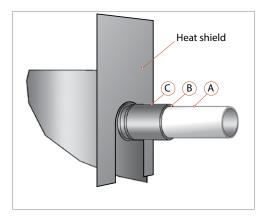
Ensure that no flux is allowed to enter into the tubing or compressor. Flux is acidic and can cause substantial damage to the internal parts of the system and compressor.
